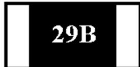
$1.96\text{K}\Omega = 196 \times 10^3 \Omega = 29\text{B}$
